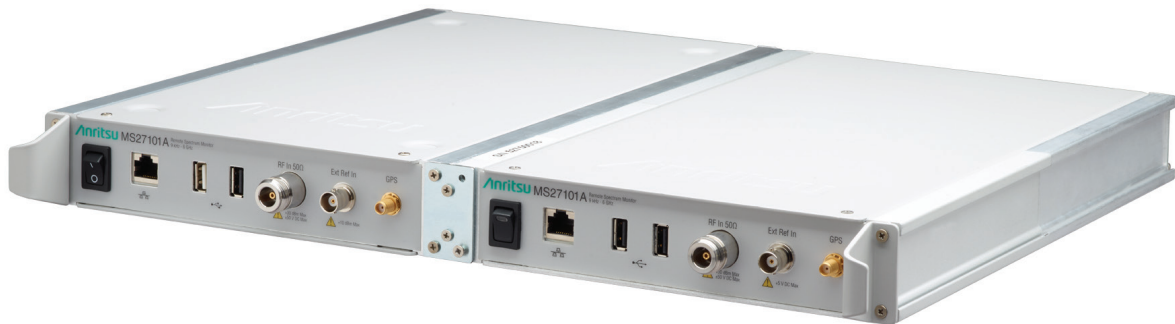
Figure 7. Two Remote Spectrum Monitor MS27101A Probes Joined Together with Bracket Kit
